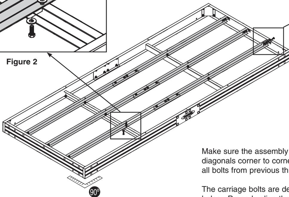
Make sure the assembly remains square by measuring both diagonals corner to corner. Once the dock is square, tighten all bolts from previous three steps.
