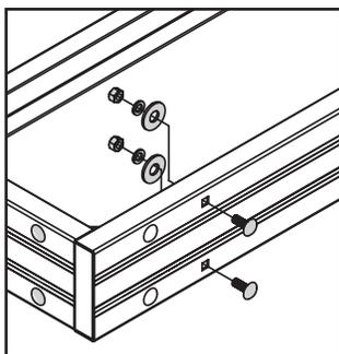
**Note:** If you purchased an accessory that needs to be bolted into the side of the dock (see accessories pages 22 and 23), you can use these exposed holes for your accessories in place of drilling new holes.
