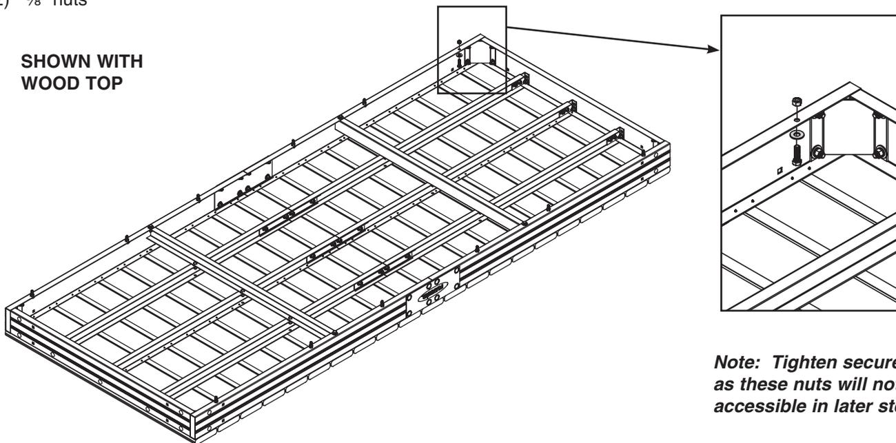
**Note:** Tighten securely as these nuts will not be accessible in later steps.
