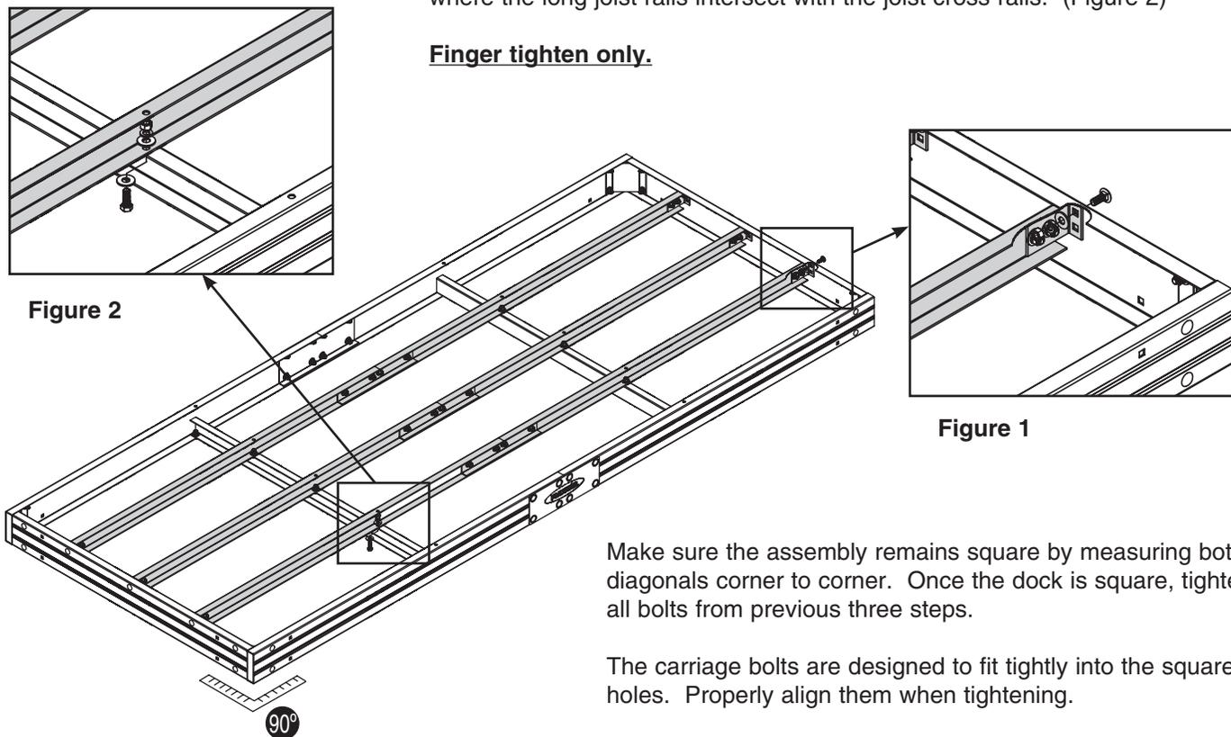
Make sure the assembly remains square by measuring both diagonals corner to corner. Once the dock is square, tighten all bolts from previous three steps.
