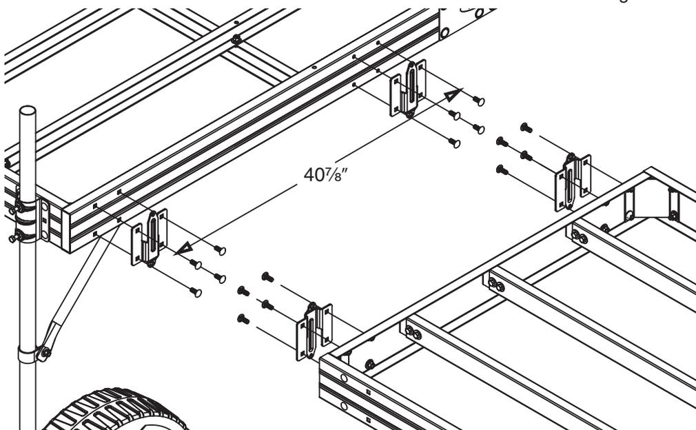
Attach the clips to the frame as you assemble the corner hardware.
