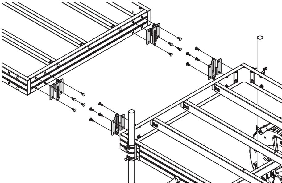
Attach the clips to the frame as you assemble the corner hardware.
