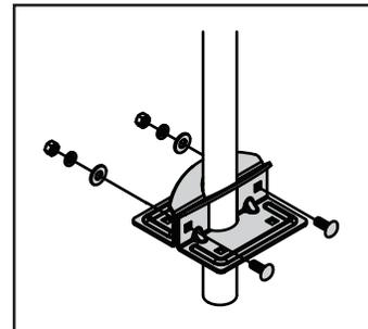
*Note: Dock pipe longer than 8 feet may require additional cross bracing.*
