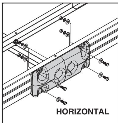
Position the bumper in desired location. For ease of assembly, you can position the bumper where you have exposed holes or replace the frame plate.
