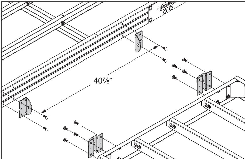
Use the long hinge (with notch) as a drill guide and mark the two hole locations. Drill  $\frac{1}{8}$ " holes through the side of the aluminum frame at the marked locations. Use the  $\frac{1}{8}$ " holes as a drill guide and drill  $\frac{3}{8}$ " holes.
