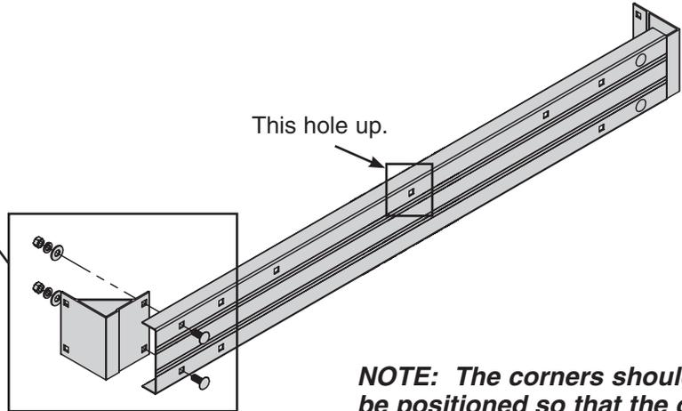
**NOTE: The corners should be positioned so that the offset sides are tight against the ends of the end frame rail.**
