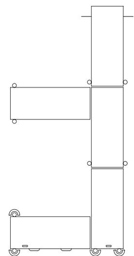
All PlayStar Docks are made from 4' x 10' modular sections which can be easily configured to meet any requirement.
