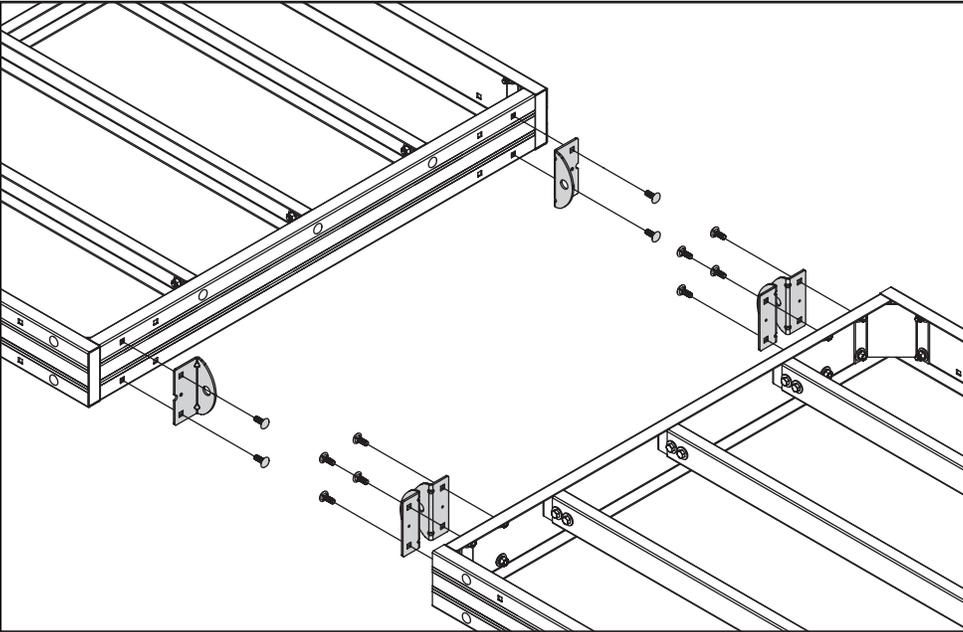
Position short hinges (no notch) pointing down in each corner of one 4' side of the next dock section to be attached.
