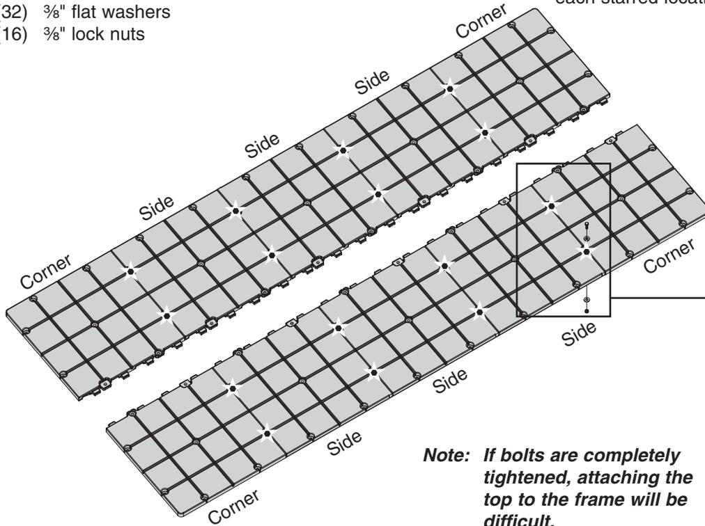
**Note:** If bolts are completely tightened, attaching the top to the frame will be difficult.
