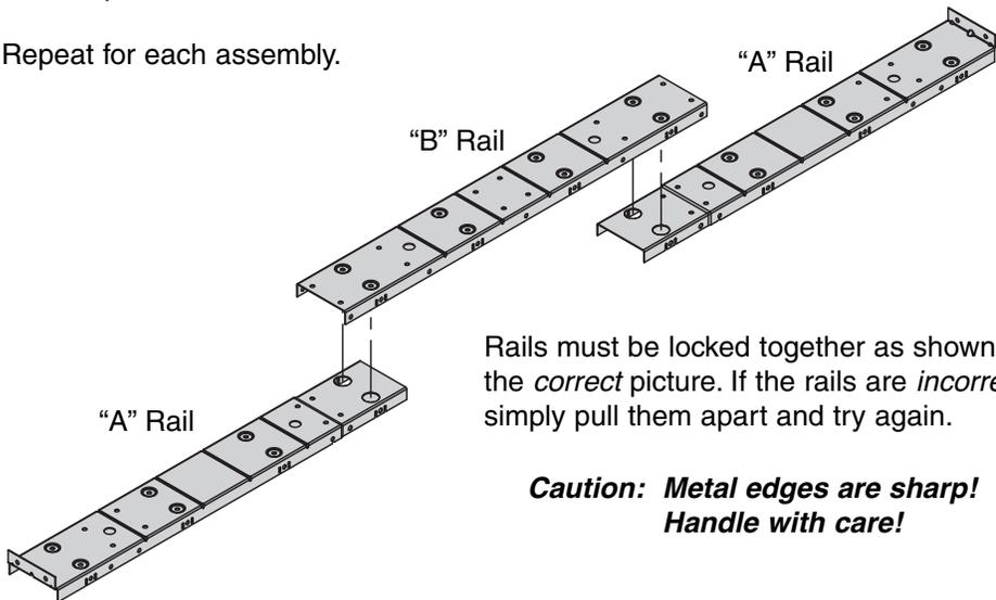
Rails must be locked together as shown in the *correct* picture. If the rails are *incorrect*, simply pull them apart and try again.
